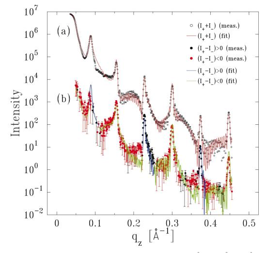
FIG. 9. (Color)  $(I_++I_-)$  (a) and  $(I_+-I_-)$  (b) intensities measured (symbols) from a Fe(34 Å)/[Gd(51 Å)/Fe(34 Å)]\_{15} multilayer near the Gd  $L_2$  edge (7929 eV). The lines represent the best theoretical fits with the model (b) in Fig. 7. Note that the colors of symbols and lines in  $(I_+-I_-)$  intensities are different for opposite signs of the intensities.
