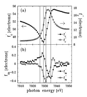
FIG. 4. Charge (a) and magnetic (b) x-ray scattering amplitudes,  $f_{c,m}$ , around the Gd  $L_2$  edge obtained from the absorption measurements for a [Gd(51 Å)/Fe(34 Å)]<sub>15</sub> multilayer. The vertical lines indicate the photon energies, where the x-ray resonant magnetic reflectivities in Fig. 5 were calculated.
