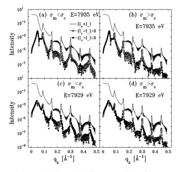
FIG. 6. Calculations with different magnetic interface roughnesses: (a) and (c)  $\sigma_m = 2.1$  Å, and (b) and (d)  $\sigma_m = 6.2$  Å. All other parameters and symbols are the same as those in Fig. 5.
