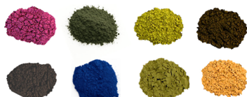
Figure 11. Images of selected samples \text{YIn}_{0.8}(\text{M}_{0.5}^{2+}\text{Ti}_{0.5})_{0.2}\text{O}_3 ( \text{M} = \text{Co}, \text{Mn}, \text{Ni}, \text{Fe} ) after heating in sealed quartz tubes (top) and after heating in air (bottom). Samples are arranged from left to right.
