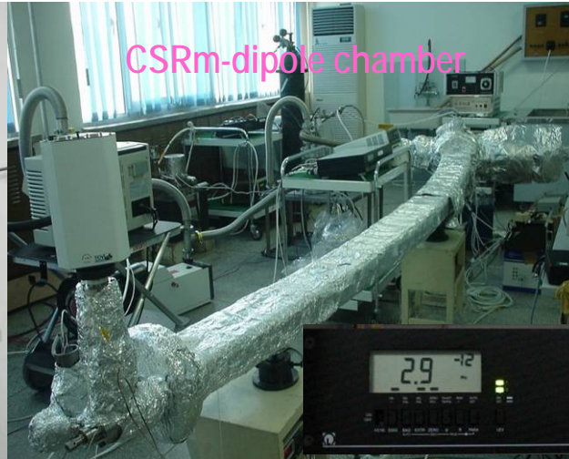
Baking jacket for dipole
