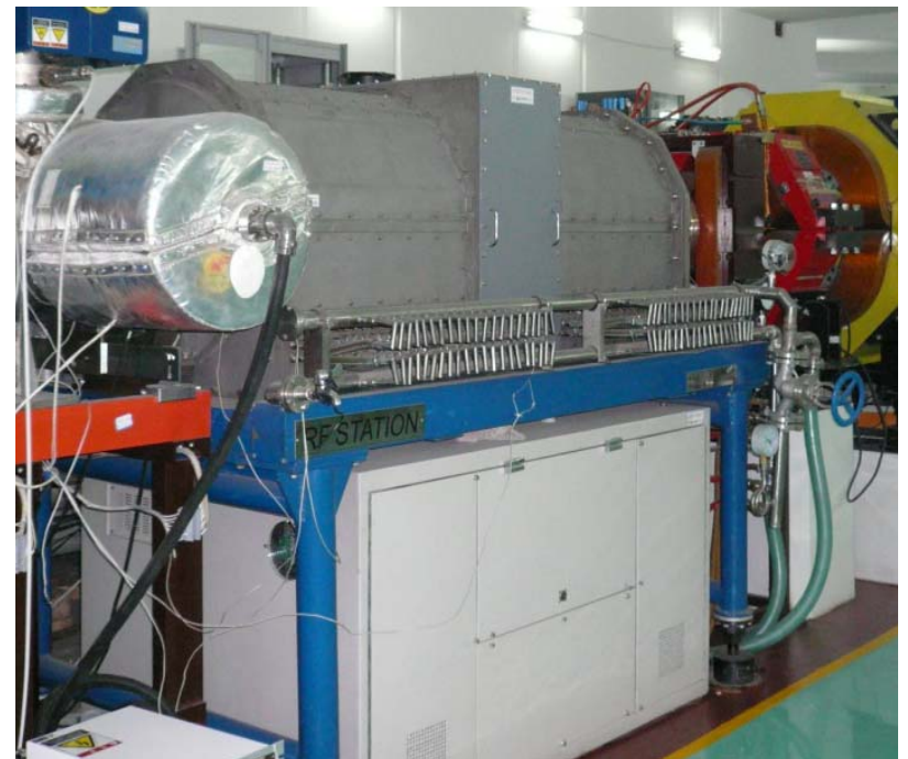
RF for beam deceleration CSR e Designed and built by IMP
