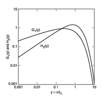
Synchrotron radiation: power given by  $G_1(y)$  brightness by  $H_2(y)$
