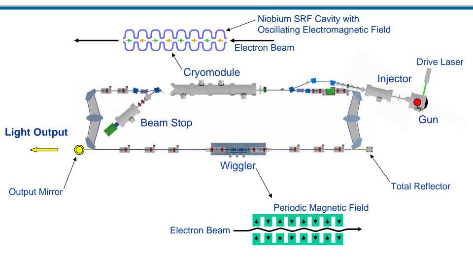
Laser Wavelength ~ Wiggler wavelength/(2Energy)<sup>2</sup>
