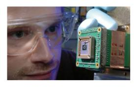
Detector for differential phase contrast imaging (S. Vogt, Sector 2), collaboration between APS-XSD X-ray Microscopy and Imaging Group and SUNY-SB/BNL.
