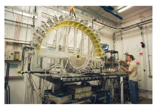
LERIX x-ray Raman scattering spectrometer at 20-ID, developed by G. Seidler and collaborators (T.T. Fister et al., "Multielement spectrometer for efficient measurement of the momentum transfer dependence of inelastic x-ray scattering," Rev. Sci. Instrum. 77, 063901 (2006)).
