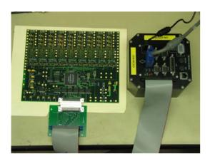
PCB electronics for testing commercial 3x3 Si APD array (contact: S. Ross)
