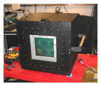
4-element fiber-optic-coupled CCD camera built by XSD-BTS (contact: T. Madden)
