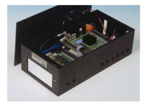
Pilatus 100K digital Si pixel array detector (SLS/PSI; XSD-BTS contact: A. Miceli)
