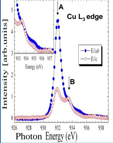
A – sensitive to the undoped sites in the  $CuO_2$ planes Cu(2,3)and to the doped  $Cu^{3+}$  chain sites (Cu(1)).
