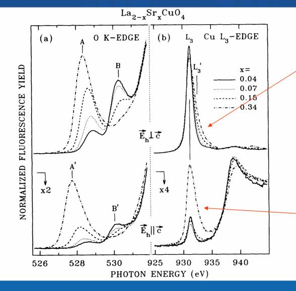
intenisty with doping Cu L<sub>3</sub> edge **Polarisation** dependence gives the symmetry of the empty d orbitals
