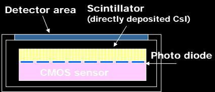
Readout 2D images pixel by pixel sequentially.
