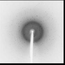
Raw diffraction image<br/>of hen egg lysozymeAfter dark current & defect<br/>pixel correctionDiffraction image recorded with CMOS
