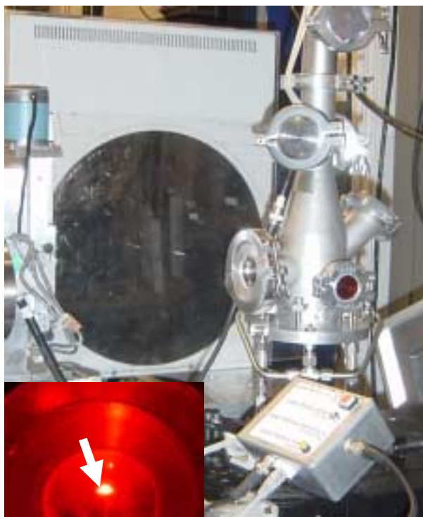
Fig. 1. Photograph of the instrument installed at the beamline. The round plate is the X-ray detector, the X-ray beam enters the chamber through the port on the right. The system was aligned by adjusting the chamber with a CeO 2 test sample located in the levitation position. The inset shows a levitated liquid sample (at arrowhead) viewed through the front port of the chamber.
