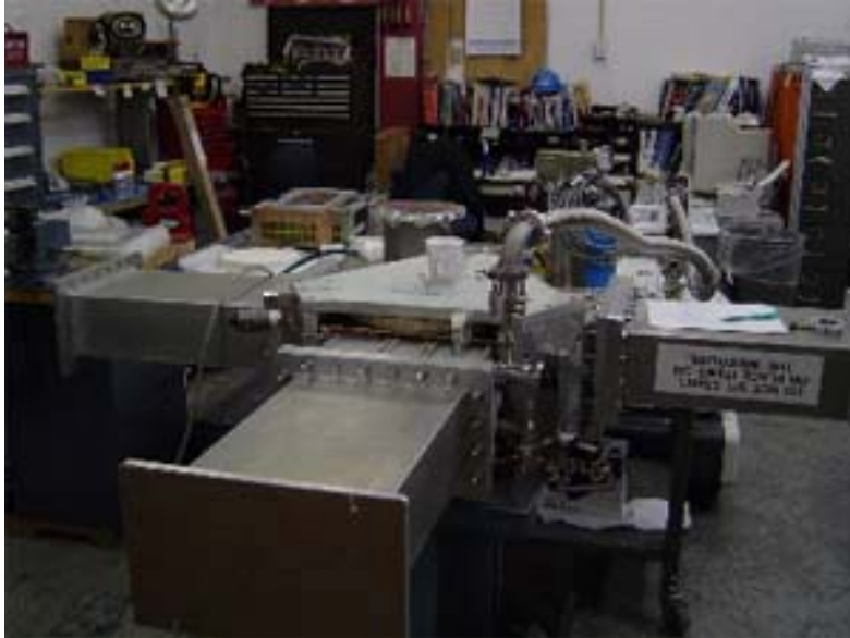
Vacuum Leak Checking a Circulator
