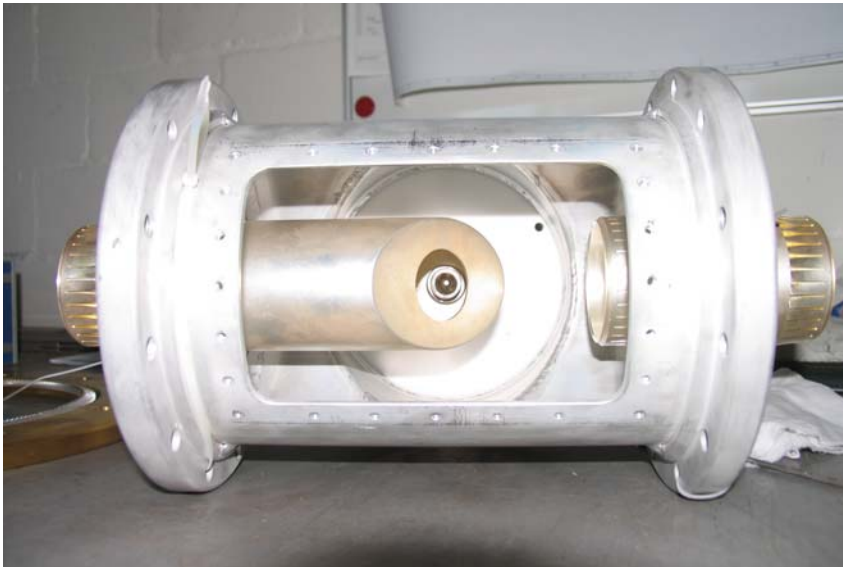
RF Switch with window opened
