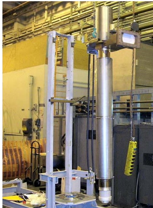
Tube sealed in shroud. Shroud facilitates fit down the bore of the magnet.
