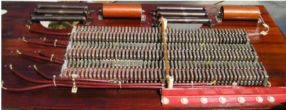
Booster RF HVPS (6 phase 47kV, 7.0A) rectifier diode stack
