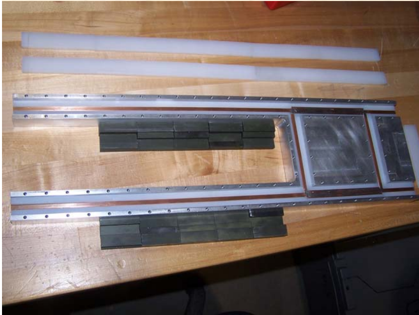
Quadrature hybrid + 2 half-wavelength tunable slabs
