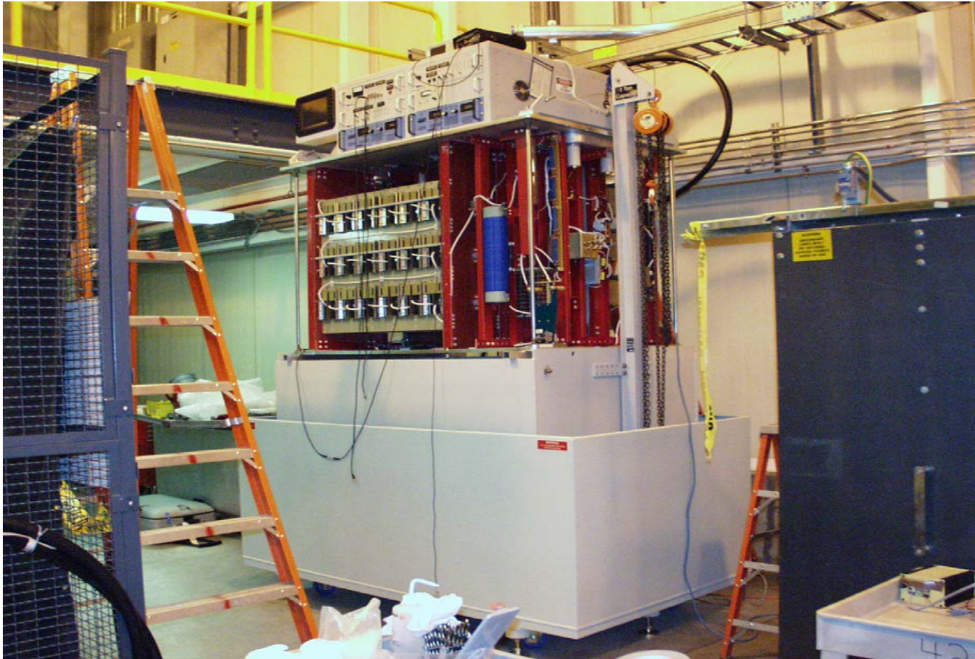
Chassis lifted from the oil tank
