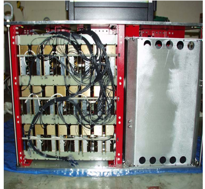
Optical connections to fast series HV output switch modules and output inductor shield
