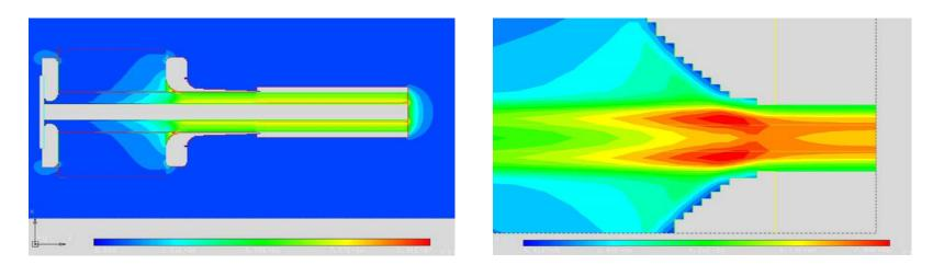
Prior to the cable manufacturing, the HV stress analysis was performed by <u>Geoff Waldschmidt</u> of the APS/ASD-RF Group for the old and new termination designs. The simulation results indicate significant drop of the peak field level inside the new connector in comparison with the old one:
