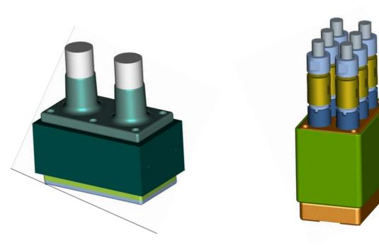
Disassembly of the G10 block and part of the magnet is required to replace one or both cables
