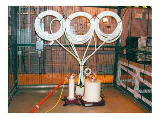
Here is a complete PAR kicker PFN cable assembly ready for testing with the PD test set.
