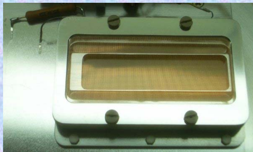
45 x 15mm cross delay line TOF detector for ion magnetic Spectrometer (Sandia/ALS)
