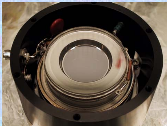
Image tube inside housing, showing the entrance window and photocathode
