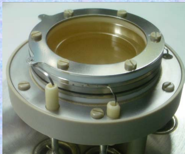
25mm Cross delay line TOF detector for electrons (UVA)
