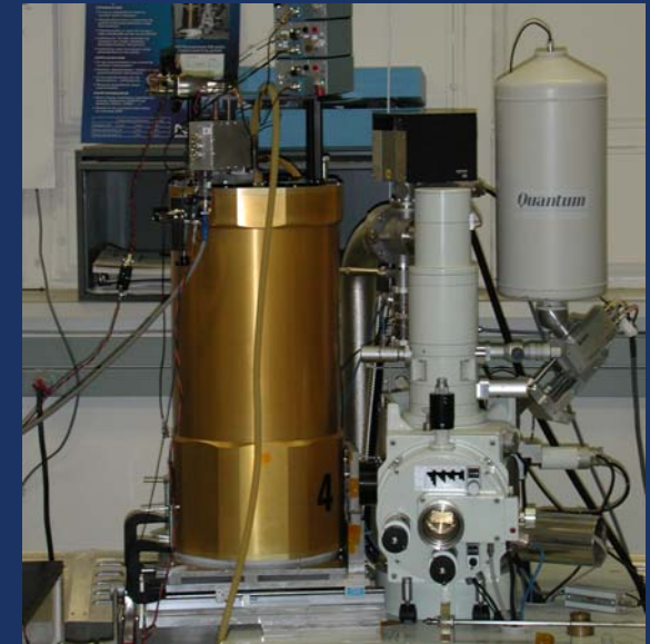
ADR and cryogen vessels mounted on SEM
