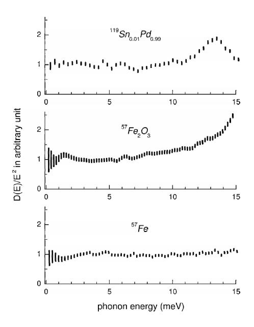
FIG. 1: The measured PDOS divided by energy squared. The size of symbols indicates the statistical error bar derived from signal counts. These samples were measured with resolutions of  $0.85 \,\mathrm{meV}$  for  $^{119}Sn_{0.01}\mathrm{Pd}_{0.99},\,0.6 \,\mathrm{meV}$  for  $^{57}Fe_2\mathrm{O}_3,\,\mathrm{and}\,1 \,\mathrm{meV}$  for bcc iron.
