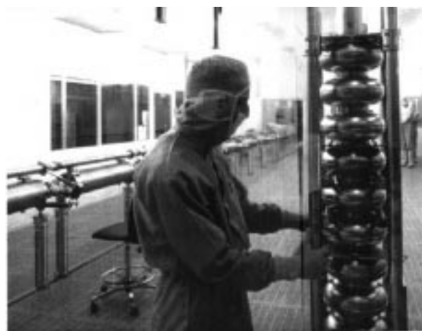
Figure 40. TTF cavity assembly in a class 100 clean room.
