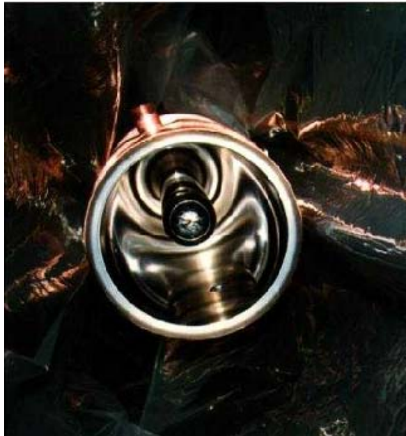
QWR Nb/Cu Cavity for CIAE 4-5MV/m at 4.2K Q_0 < 10^9
