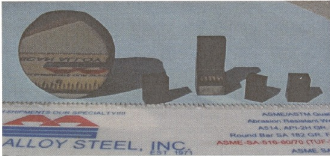
Figure 7. Examples of machined samples from HIPed magnesium diboride. Notice mirror like quality of polished sample on left and third from left. Three small parallelepipeds with sharp corners were machined for high accuracy RUS measurements of elastic constants.
