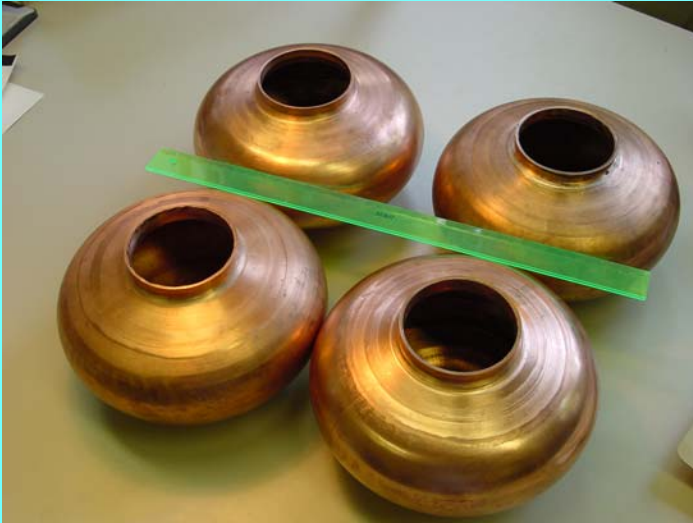
Single cell NbCu cavities produced at DESY by hydroforming from KEK sandwiched tube.
