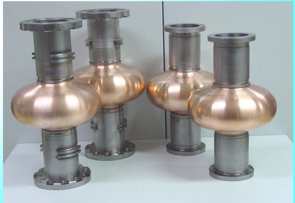
Single cell NbCu cavities produced at DESY by hydroforming from KEK sandwiched tube.
