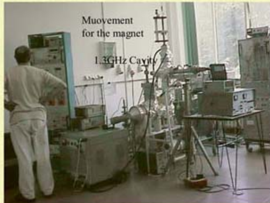
The laboratory setup in Swierk in which the UHV system equipped with a cylindrical arc source shown in the photograph has been recently put into operation.
