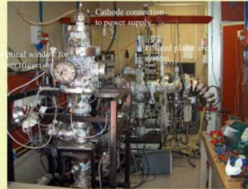
Laboratory in Rome: Cylindrical arc system and planar filtered arc
