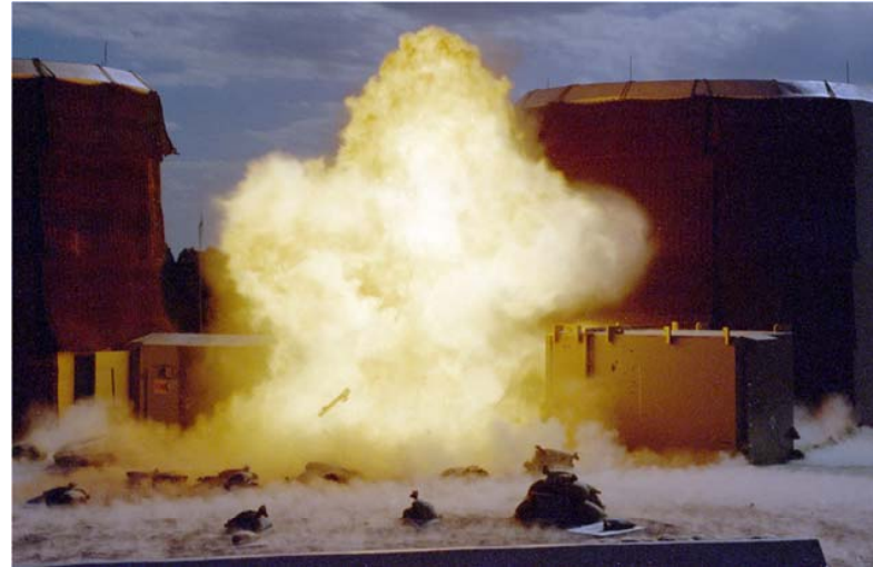
A "hydrotest" on the operational first axis of DARHT
