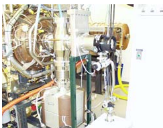
Storage Ring RF Cavity Vacuum System.
