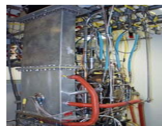
Single-Cell RF Test Cavity Assembly.
