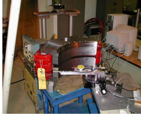
Fig. 3b: The field and thermal test setup includes magnet, probes, recorder on table.
