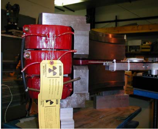
Fig. 3a: The Hall probe setup at center of poles' gap, water channels on 3 coils.
