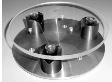
Fig. 1: 3-V groove kinematic mount.
