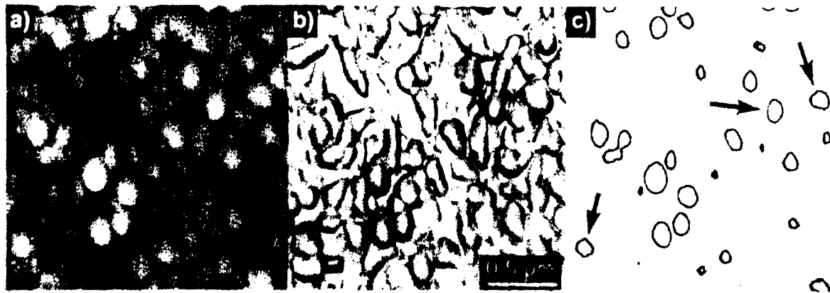
Fig. 4. AFM images at the coverage corresponding to Te/Mo = 1.6: (a) half-tone image, (b) 3d-rendered image, (c) contour plot (arrows indicate grain of nearly hexagonal symmetry).
