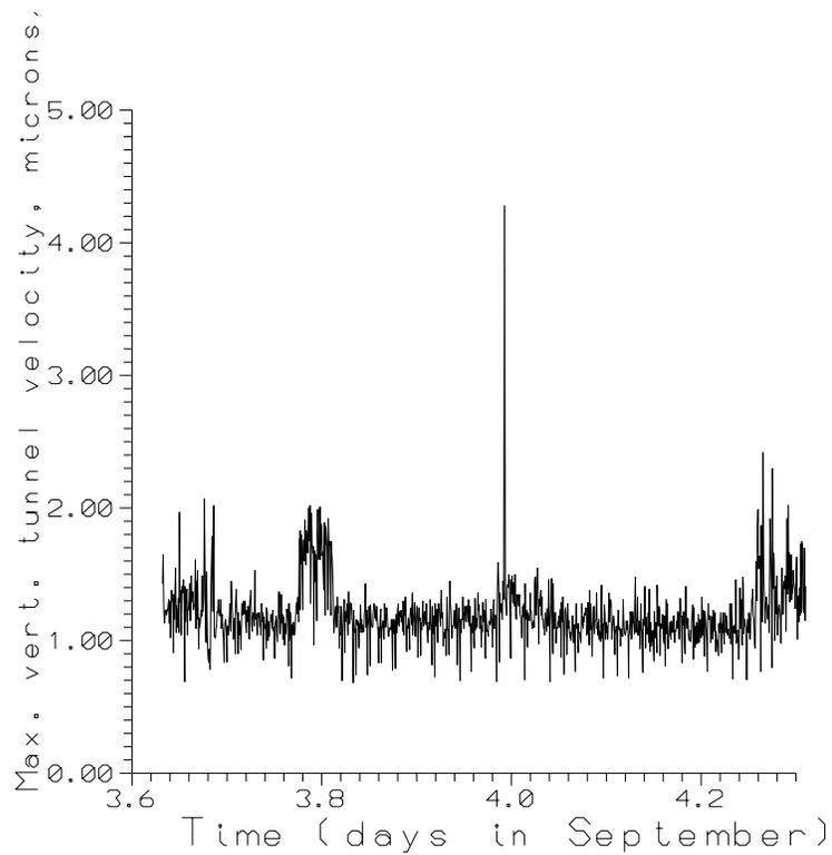
Figure 10: Vibration amplitudes in the tunnel of Tevatron over 16 hours starting 3:30pm 09/03/1997. The Main Ring and the Tevatron ring are under operation.
