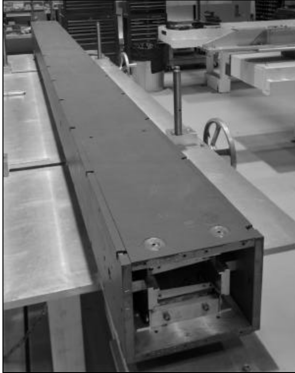
Figure 9. Assembled gradient magnet showing the survey fiducials
