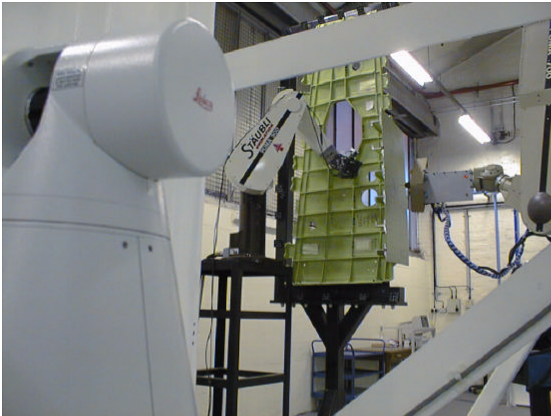
Fig. 7 View from tracker towards internal and external robots on either side of test piece
