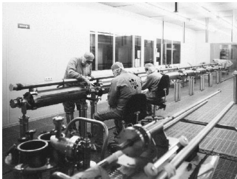
Figure 4: Connecting the cavity string in the cleanroom
