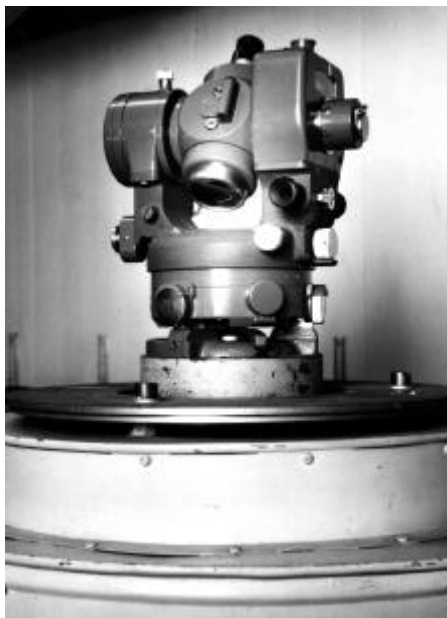
Figure 6: Kern theodolite on pillar
