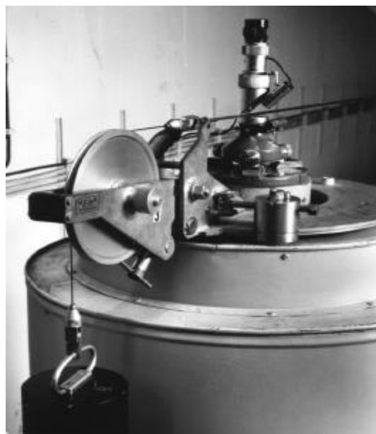
Figure 4: Invar tape measuring device
