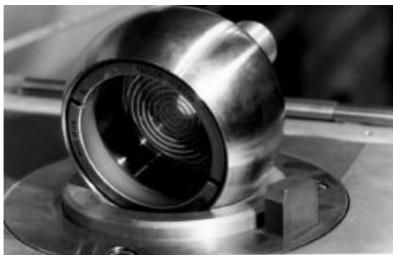
Figure 25: Taylor Hobson sphere on HERA-socket
