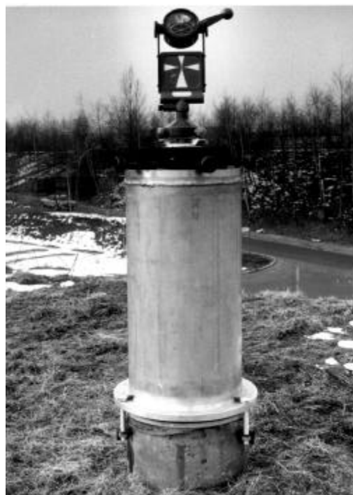
Figure 19: Survey pipe above the PETRA-tunnel
