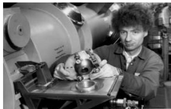
Figure 26: Survey platform with centering support for theodolite
