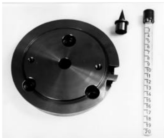
Figure 11: Reference plate for beam line magnets
