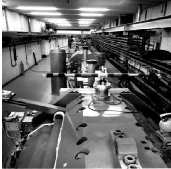
Figure 16: Straight section DORIS with 1m-scale bar on interaction quadrupole
