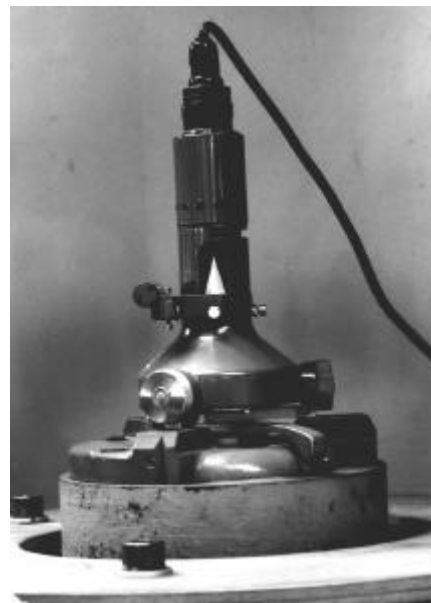
Figure 7: Target for horizontal angle measurements
