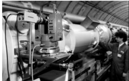
Figure 28: CCD - camera behind the theodolite
