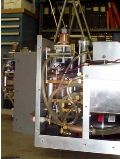
Fig. 3 Internal view of master unit, pump at lower right
