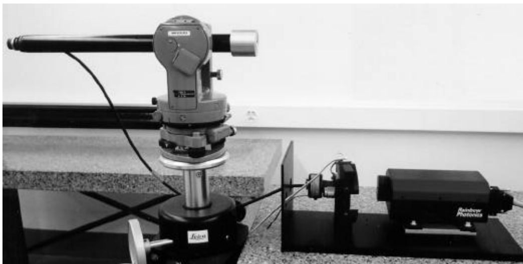
Fig. 2 Schematic drawing and realization of the ETH-dispersometer light source
