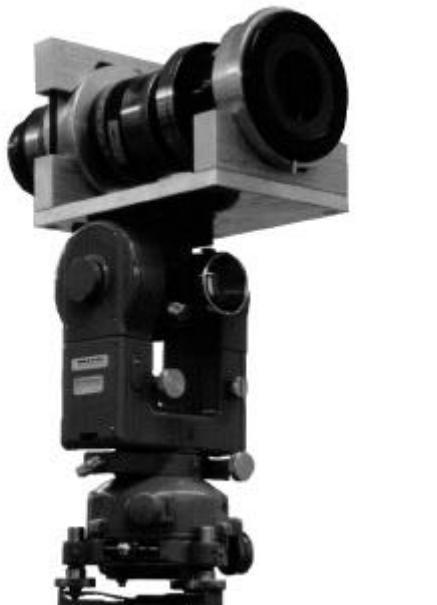
Fig. 4 Dispersion telescope mounted on a WILD T2 theodolite, additionally the dispersion telescope is rotatable around its optical axis.
