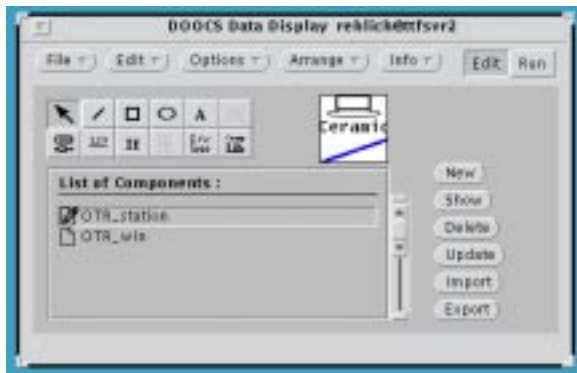
Figure 1. Main window of the ddd editor. The 'OTR station' is selected and shown in the small preview window.
