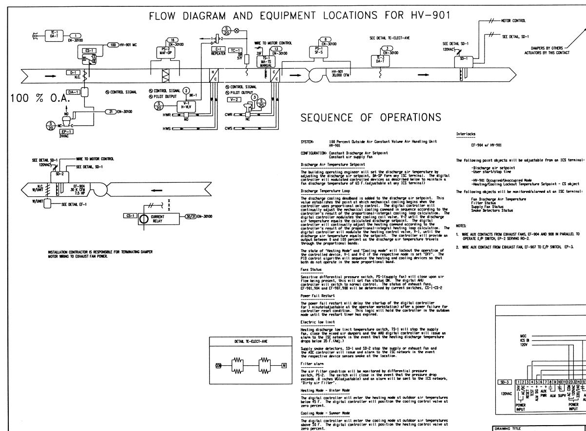
DEVICE TAG GTY CODE NUMBER DESCRIPTION SEE DAMPER SCHEDULE SEE DAMPER SCHEDULE D-1-3 VALVE, SOL.AIR, 3-VAY END SVITCH SENSITIVE DIFF PRES CTL REMOTE HTD PROBE V-2410-2 802T-CVP P32AF-2C FTG18A-600R CS-1 705-ND CURRENT SVITCH-VERIS DUCT DETECTOR, ION, SAMPLING TUBE FOR RESET/TEST SENSOR, 1000 OHM +/- .25X HOUSING F/O O.A. TEMP. TEMP SENSING ELEMENT 17' SD-1-SD-3 DH400ACDCI ST-10 RTS-451 TE-1 TE-6001-2 TE-6100-1 TE-3 TEMP CONTROL 4 VIRE, 2-C
